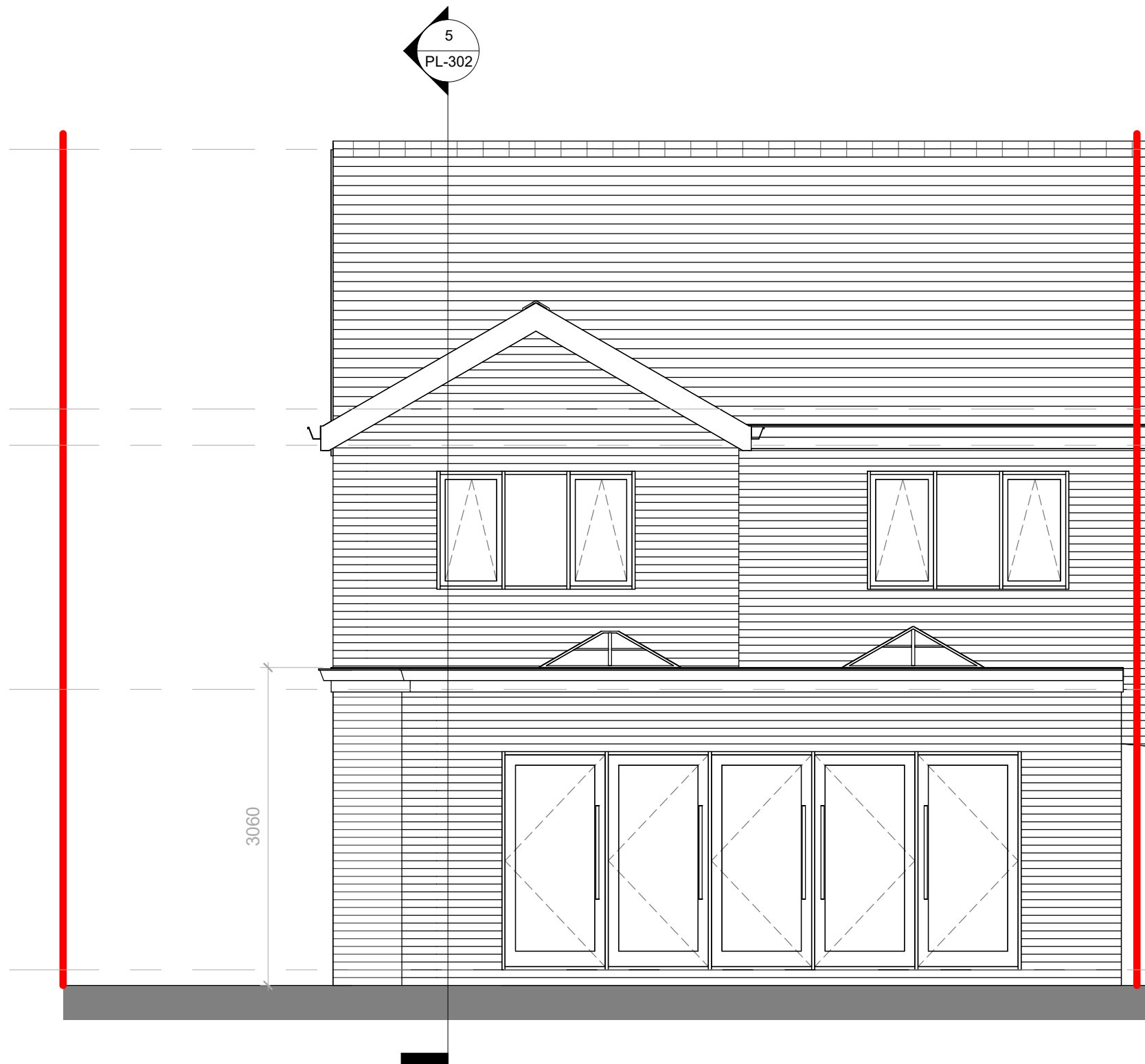
3 As Proposed Rear Elevation 1 : 50
