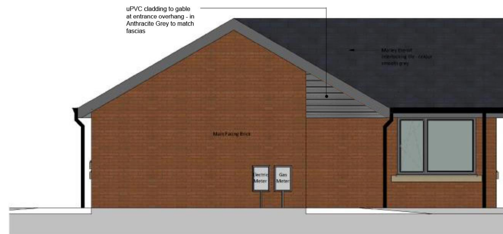
04 Gable Elevation 2 Brick Type A 1 : 50
