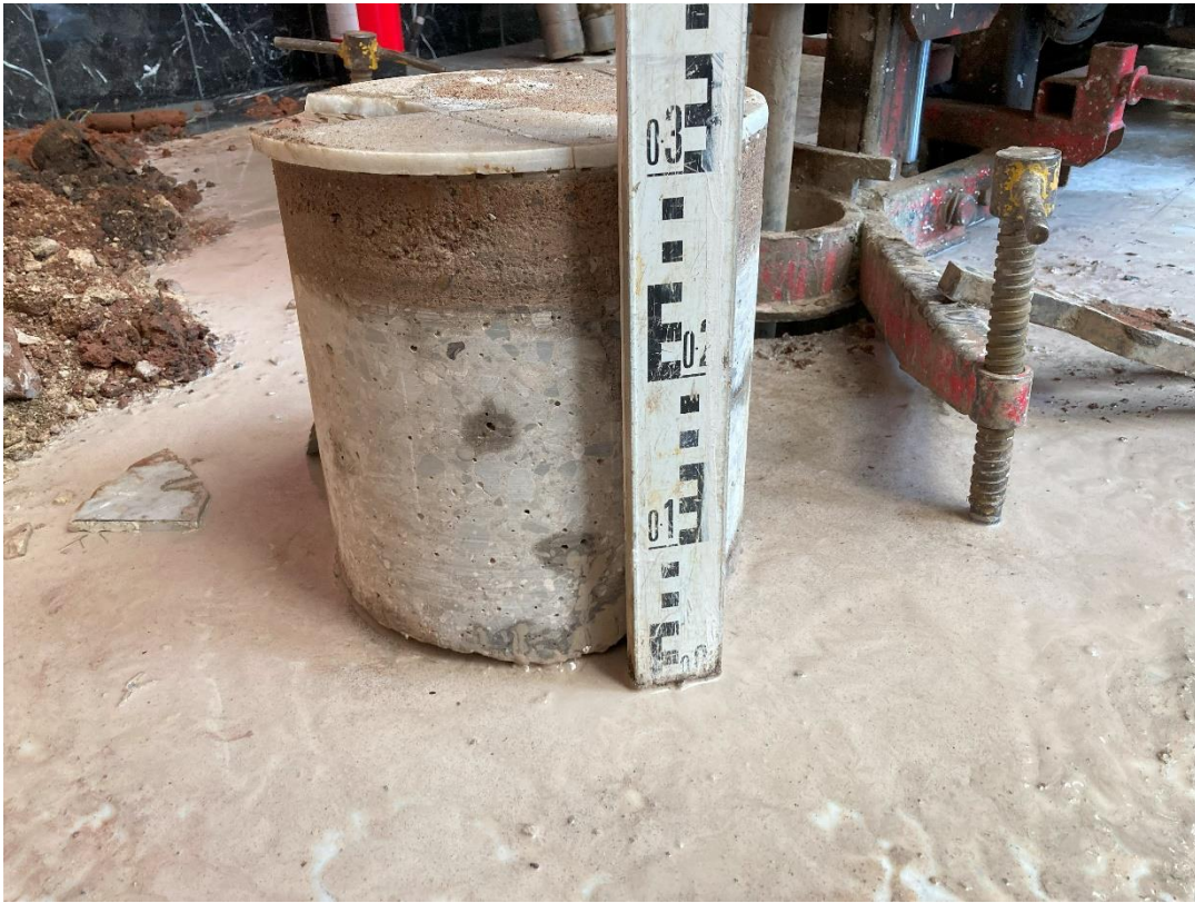
Plate 3 – WS02 concrete core, gl to 0.32m bgl.
