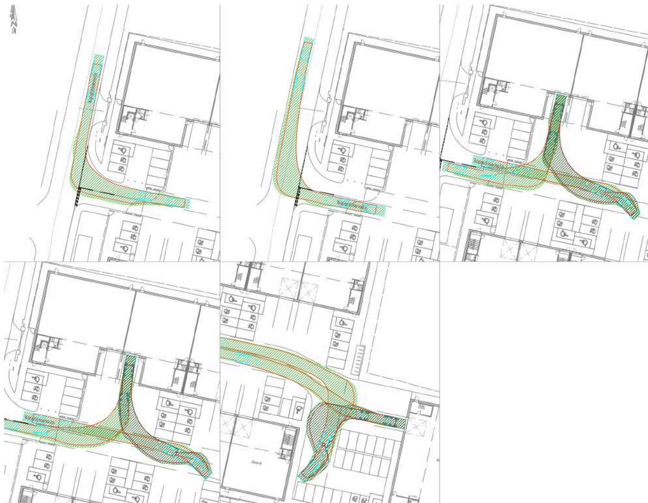
Figure 3.3 : Swept Path Analysis – 16.5m Articulated HGV
