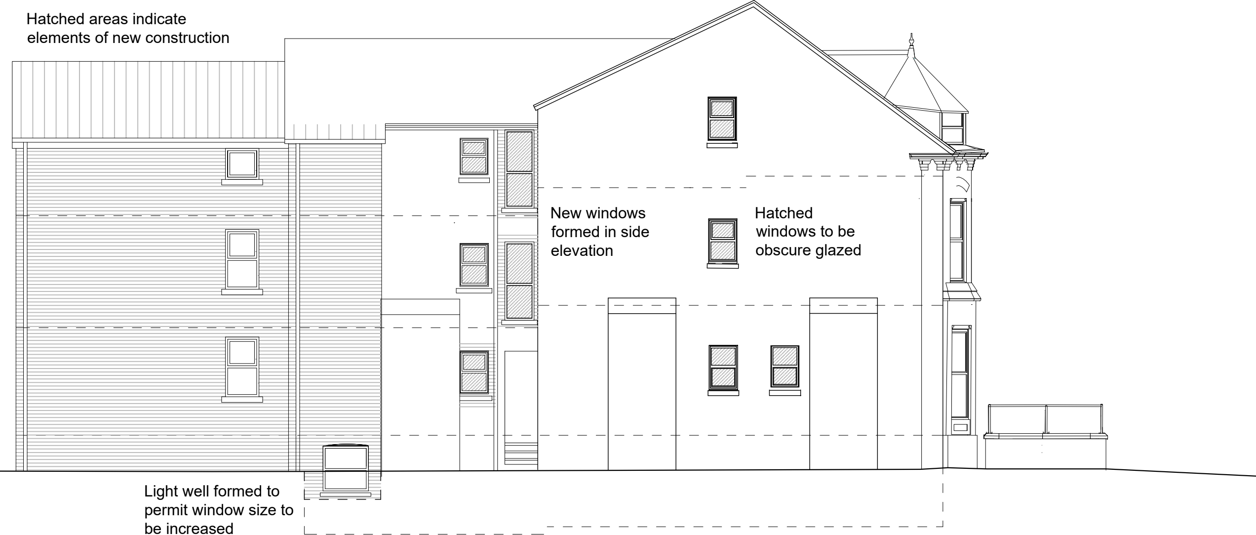
Side Elevation (North)
