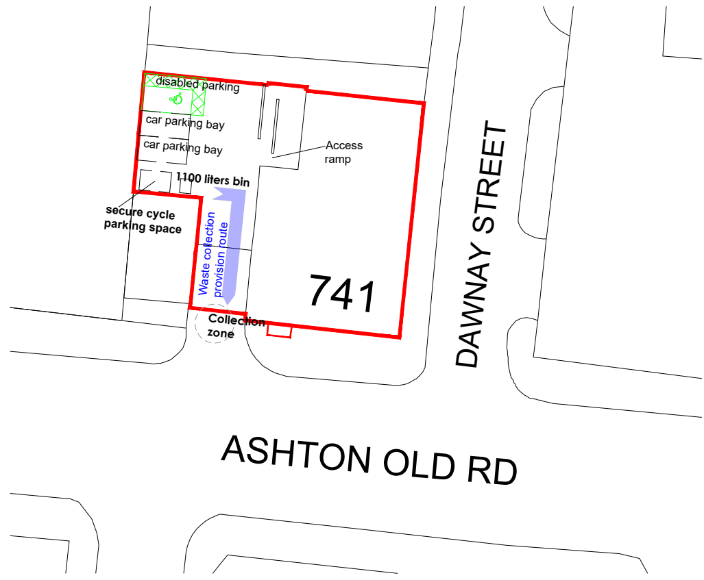
Proposed Site Plan 1:500@A3
