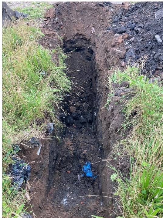
PLATE 6 EXAMPLE OF SHALLOW GRANULAR MADE GROUND (TP106)
