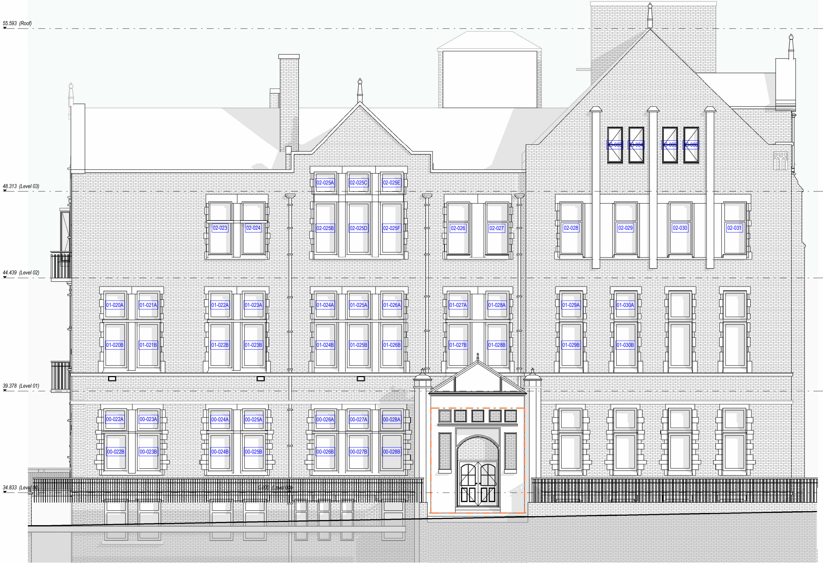
1 Proposed Glazing Window Alterations_South Elevation 1 : 100
