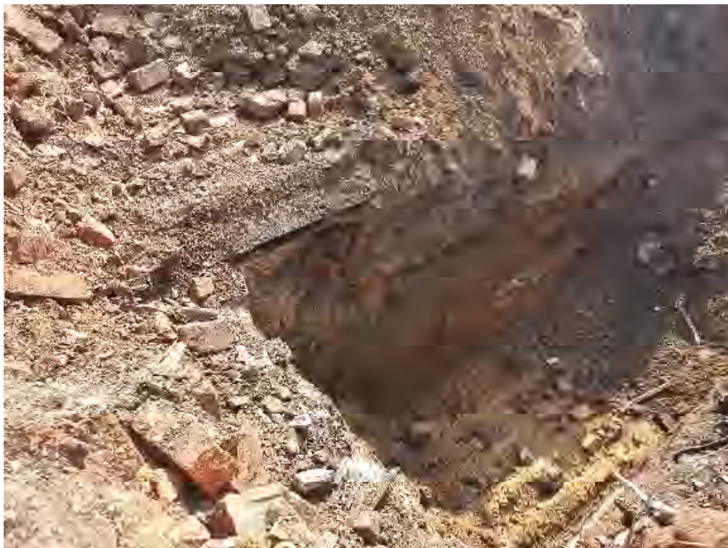
Photo No. 4: TPI02 – Made Ground / natural horizon
