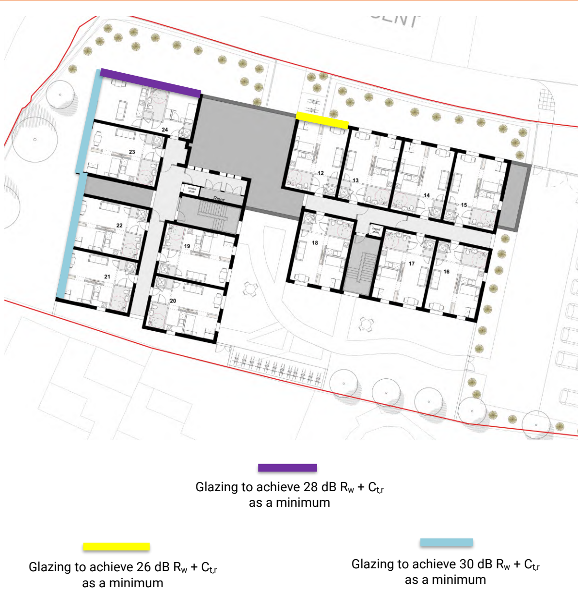
FIGURE 5.2 LOCATION OF HIGHER SPECIFICATION GLAZING (FIRST FLOOR)
