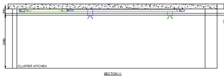
Figure 25 – Sections of Typical Vertical MVHR Layout Option 2B – Individual MVHR Unit Serving Cluster Kitchen
