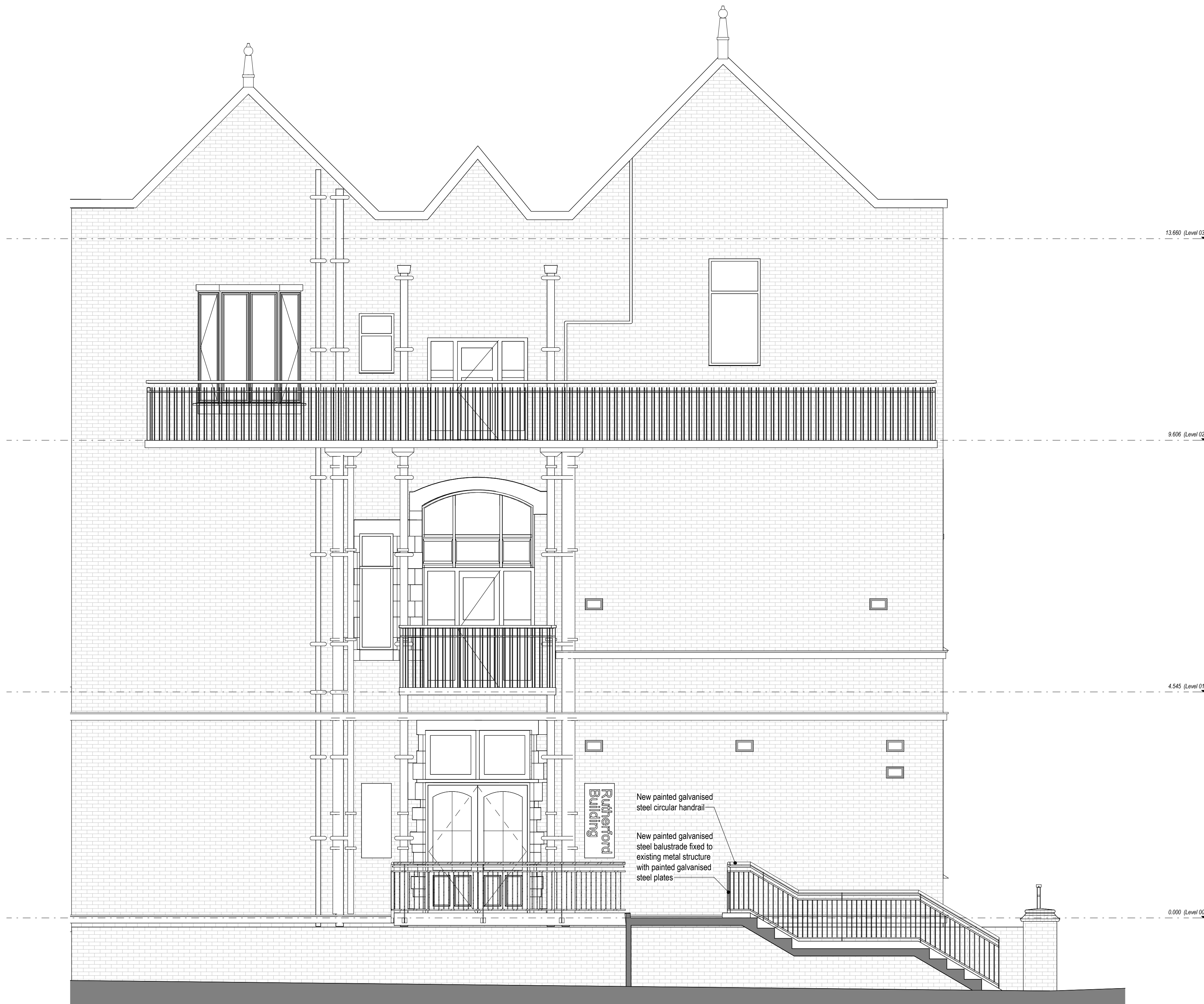
2 Entrance Ramp & Stairs Elevation A 1 : 50
