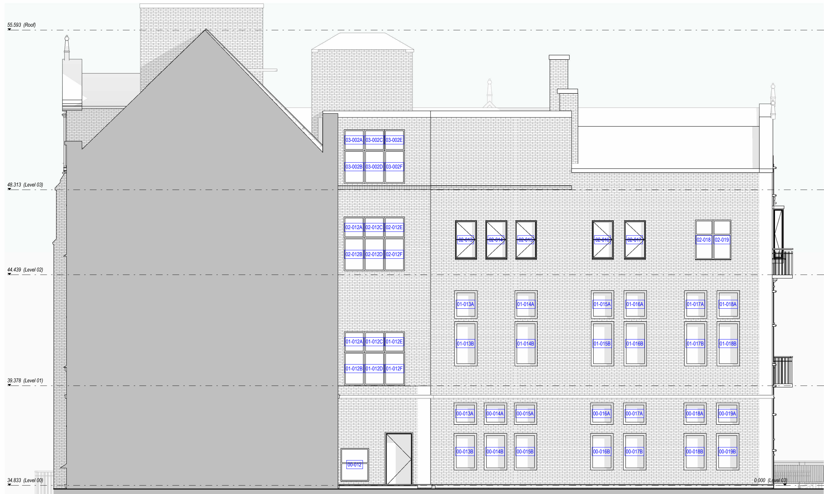
1 Proposed Glazing Window Alterations_North Elevation 1 : 100
