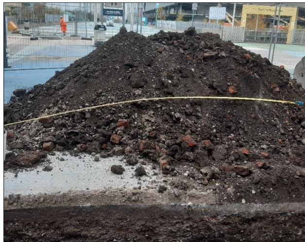
Figure 4-3 Dark brown material located beneath Type 1-style material contains abundant brick and concrete with rare metal and occasional slag.
