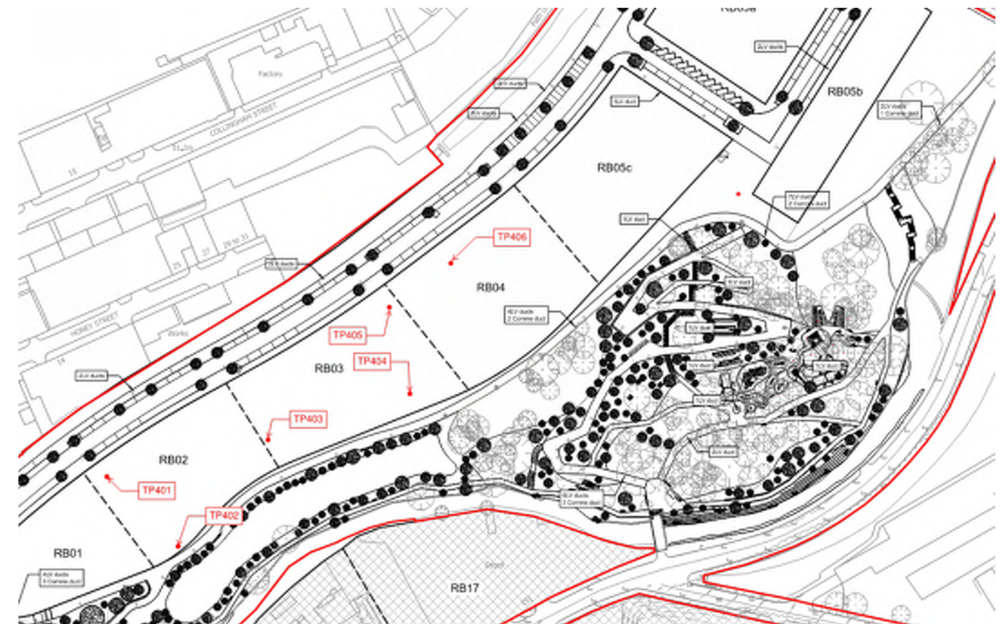
Figure 5: Initial PFAS ground investigation (January 2023) - trial pit locations
