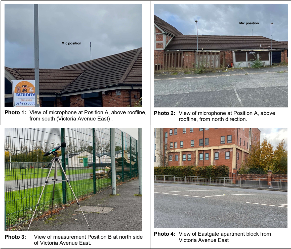
Figure 2: Photos showing measurement positions at defined receptor locations.
