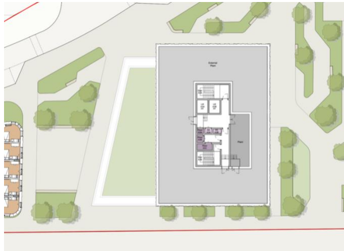
Figure 7.4 - Building A3 Roof Enclosure
