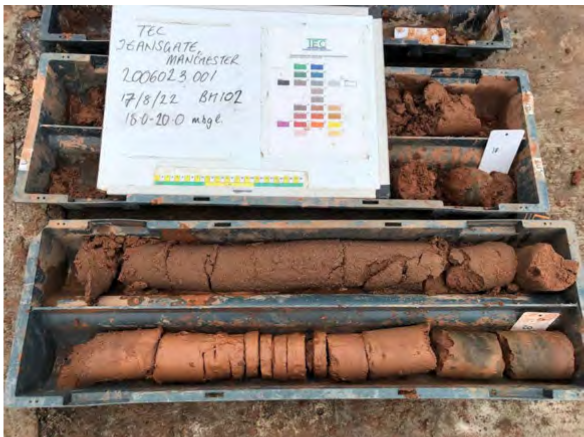
Photograph 8: View of sand/sandstone recovered from 18.0 to 20.0mbgl in BH102.
