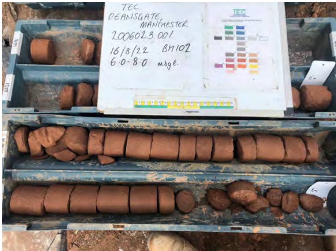
Photograph 7: View of sandstone recovered from 6.0 to 8.0mbgl in BH102.
