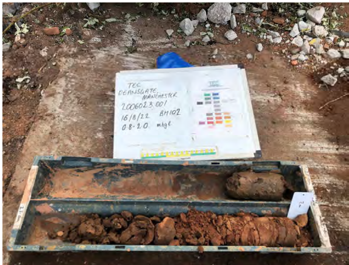
Photograph 6: View of materials recovered from 0.8 – 2.0mbgl in BH102.
