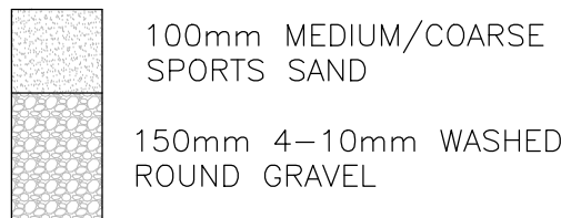
SECONDARY DRAINAGE DETAIL (1:10)
