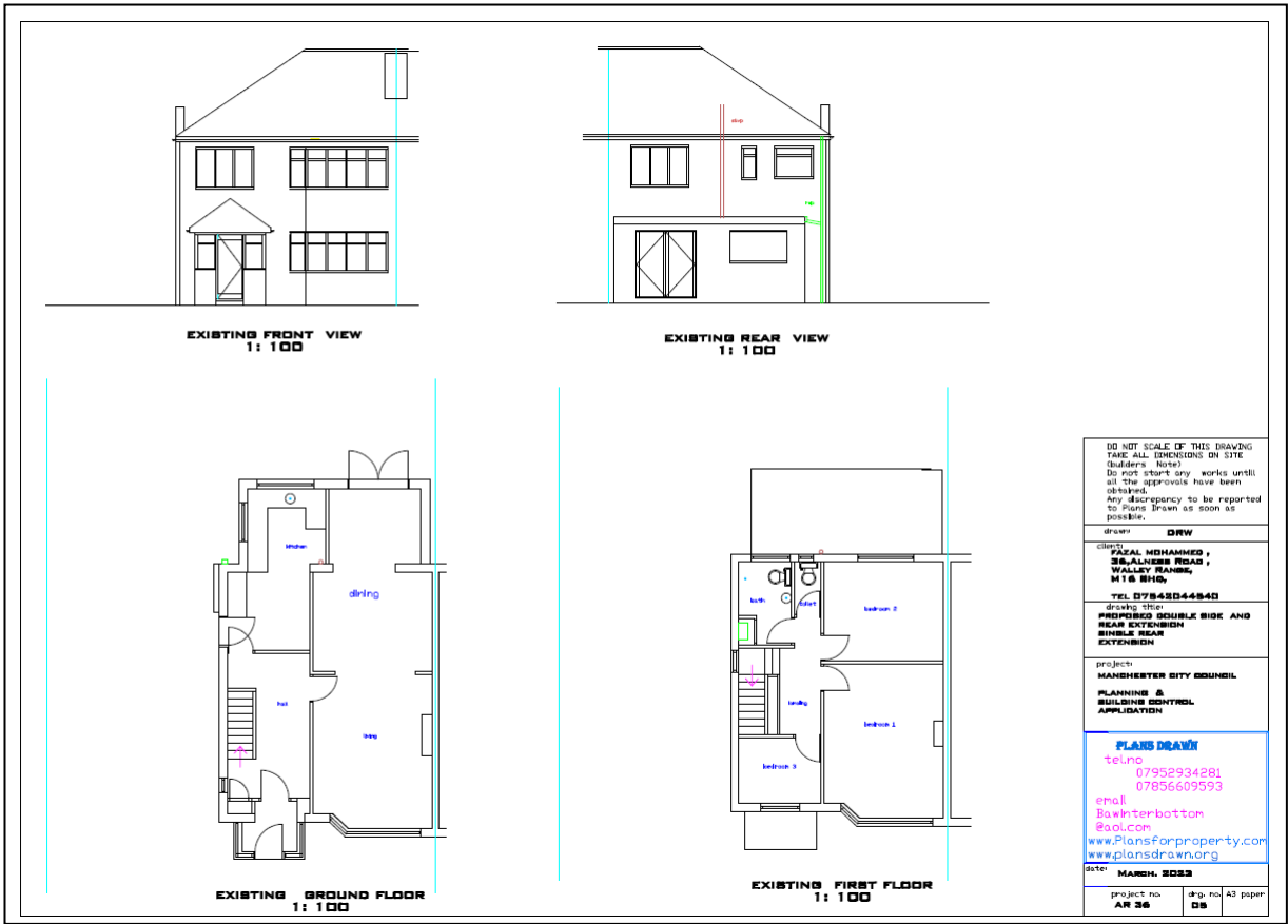
Figure 5. Existing Elevations and Floor Plans
