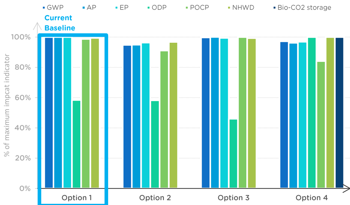
Figure 9. Normalised comparison of BREEAM Mat01 options for all BREEAM impact categories (GWP – Global Warming Potential, AP – Acidification Potential, EP – Eutrophication Potential, ODP – Ozone Depletion Potential, POCP – Photochemical Ozone Creation Potential, NHWD – Non-Hazardous Waste Disposed).
