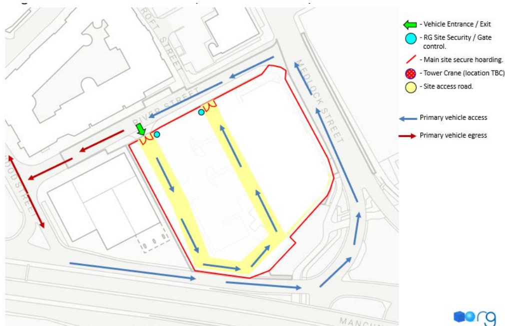
Figure 4.2 Primary access and egress routes
