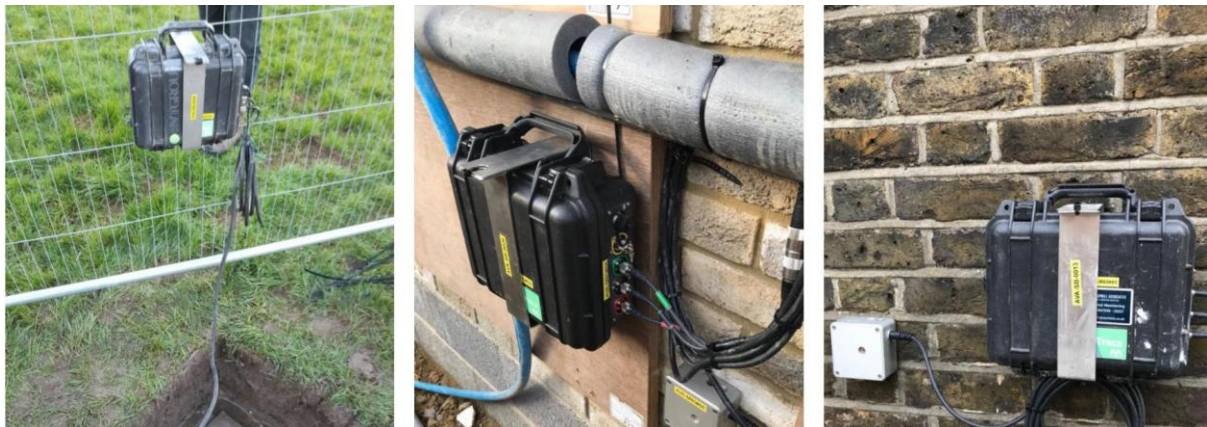
Example of vibration monitoring equipment
