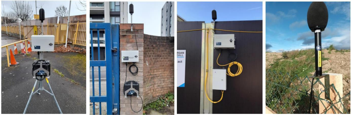
Example of noise monitoring equipment
