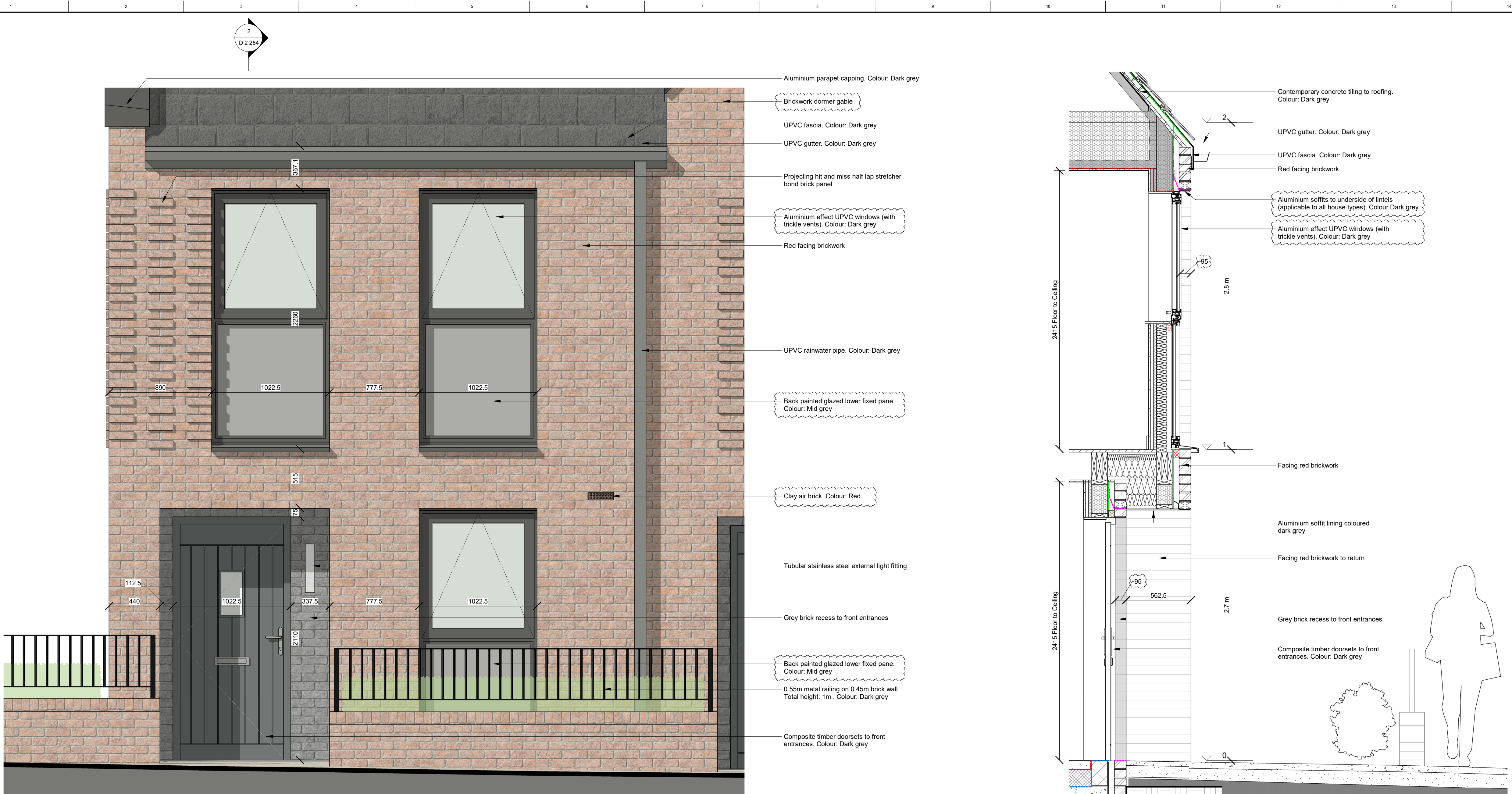
1 Typical House Facade: Elevation 1:20
