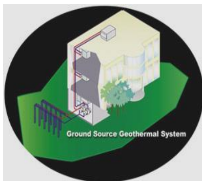
Ground Source Heat Pump Installation
