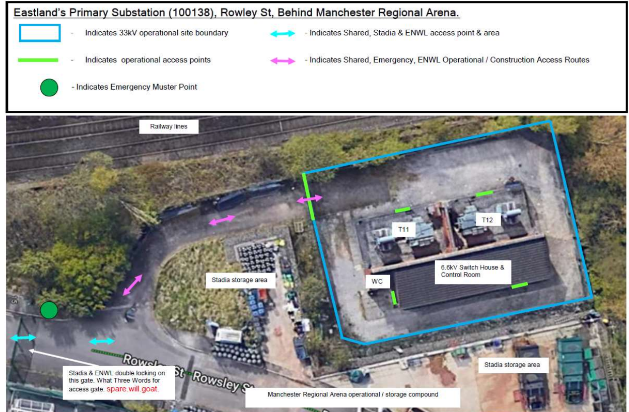
Fig 2: Substation constraints plan:
