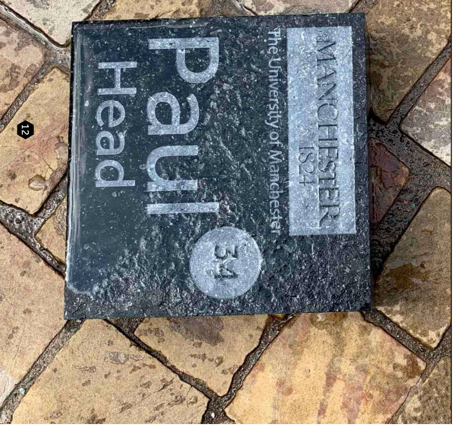
SAMPLE OF PROPOSED KILKENNY BLUE FLAMED LASER ETCHED PAVERS; PHOTO OF STONE WET
