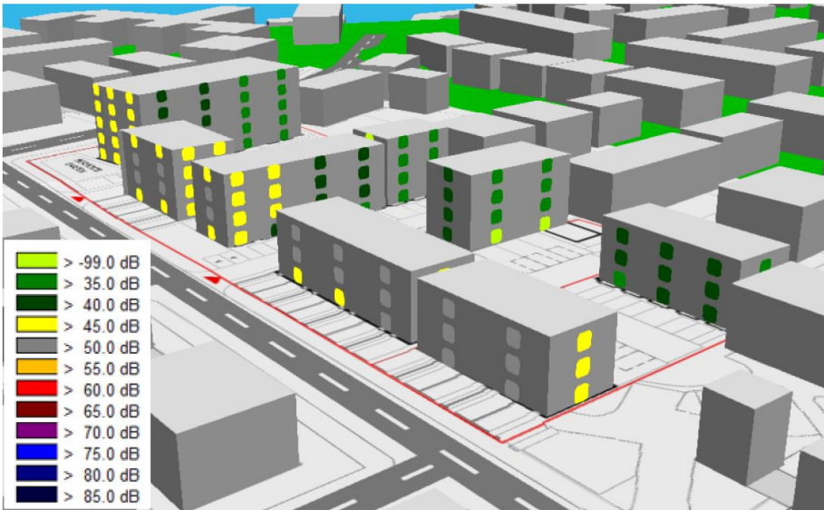
Incident Noise Levels –Daytime looking north.
