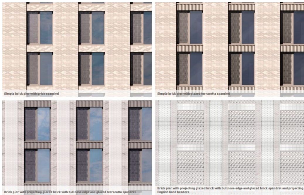
Figure 4.3: Typical detailing of York Street elevation
