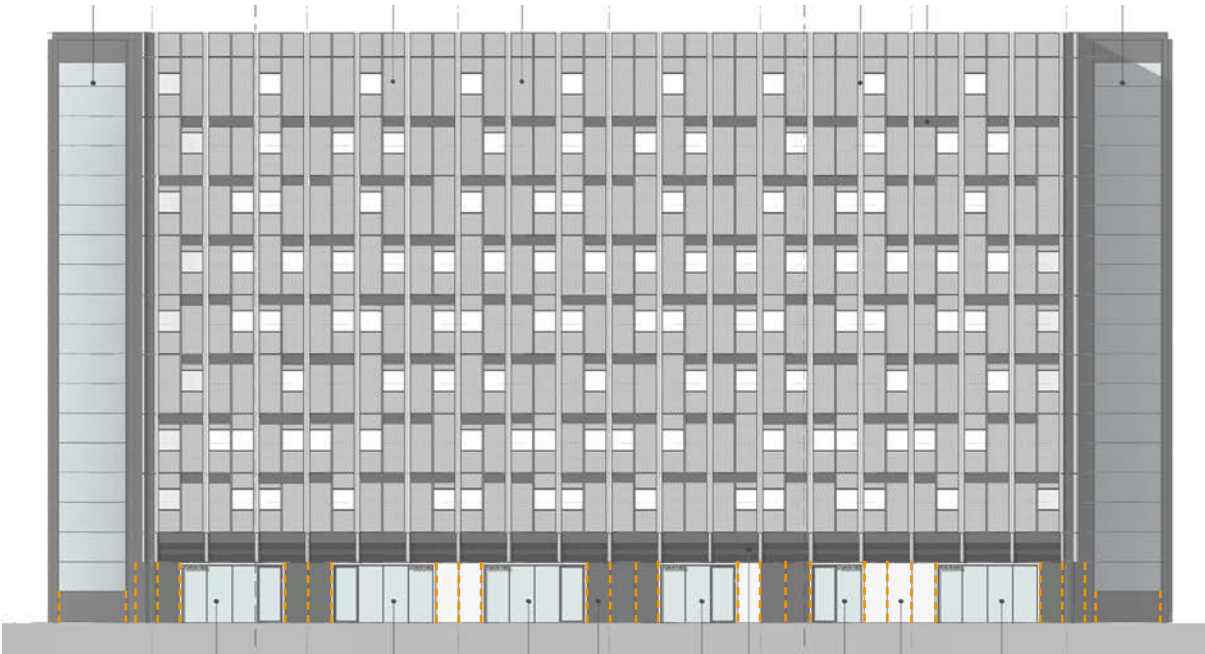
Joints to be concealed with capping
