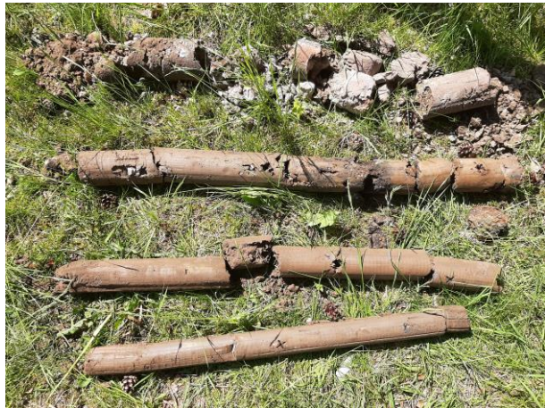
Photograph 4: Cores recovered from BH4.
