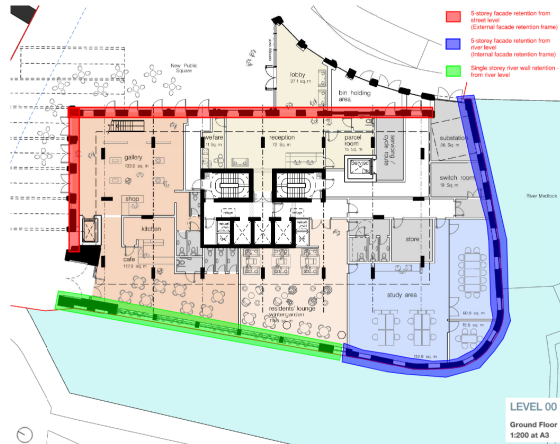
Figure 6: Facade Retention Plan, Civic Engineers.
