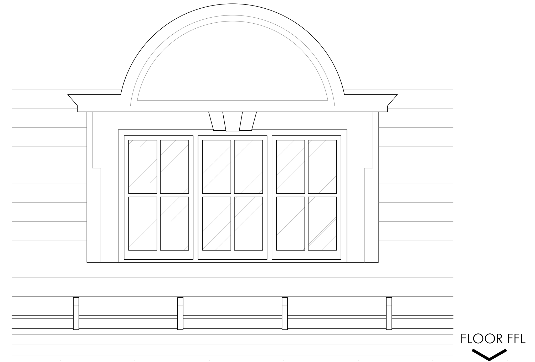
TYPICAL FOURTH FLOOR FRONT EXTERNAL WINDOW ELEVATION SCALE 1:20
