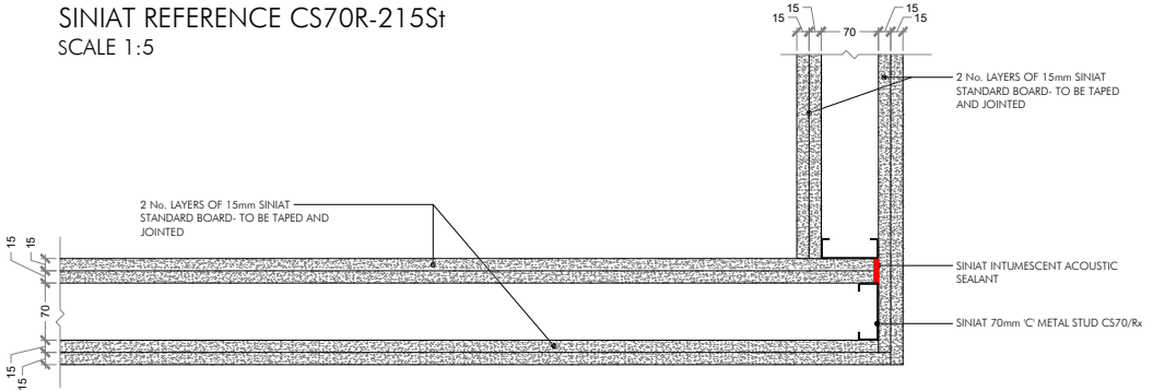
PLAN DETAIL DT04 TYPICAL PARTITION 'TYPE A' 90 DEGREE CORNER SINIAT REFERENCE CS70R-215S† SCALE 1:5
