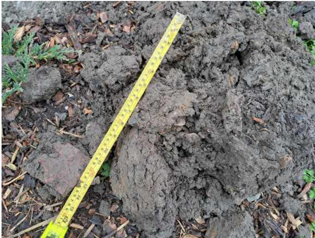
Photograph 16 VP03 cover system topsoil.
