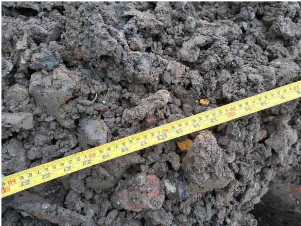
Photograph 20 VP04 showing subsoil comprising cover system.
