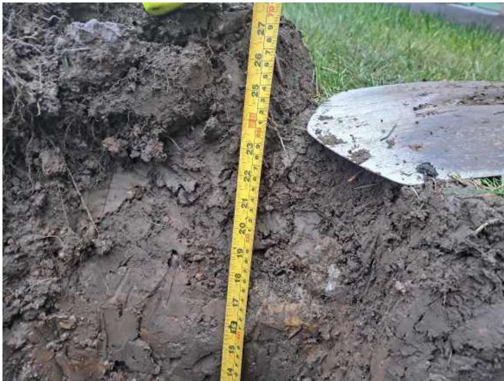
Photograph 22 VP05 showing thickness of cover system.
