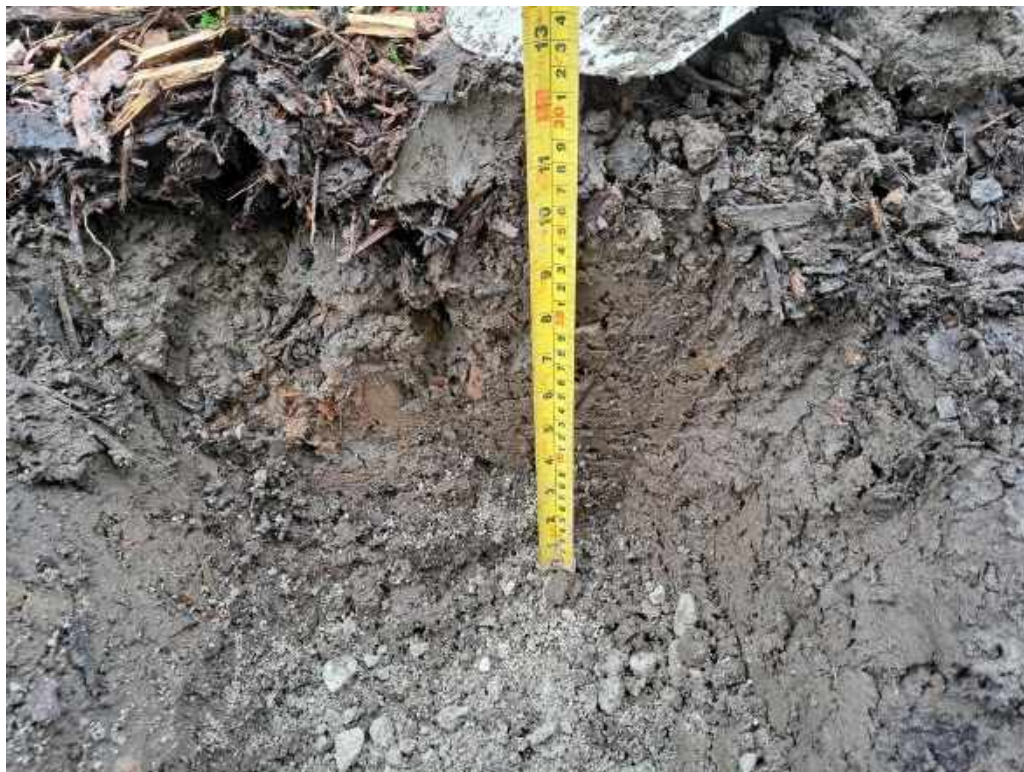
Photograph 14 VP03 showing thickness of cover system.
