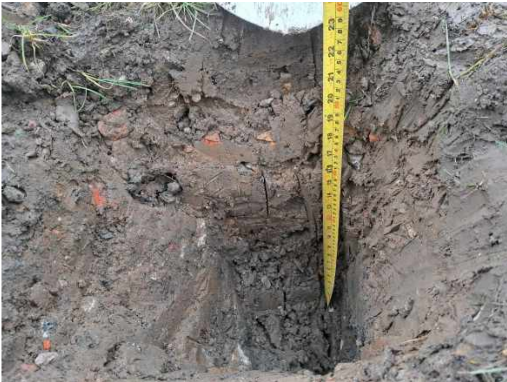
Photograph 18 VP04 showing thickness of cover system.
