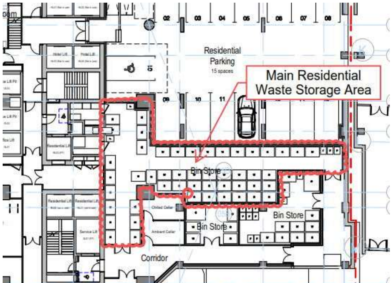
Figure 2-5: Main Residential Waste Store
