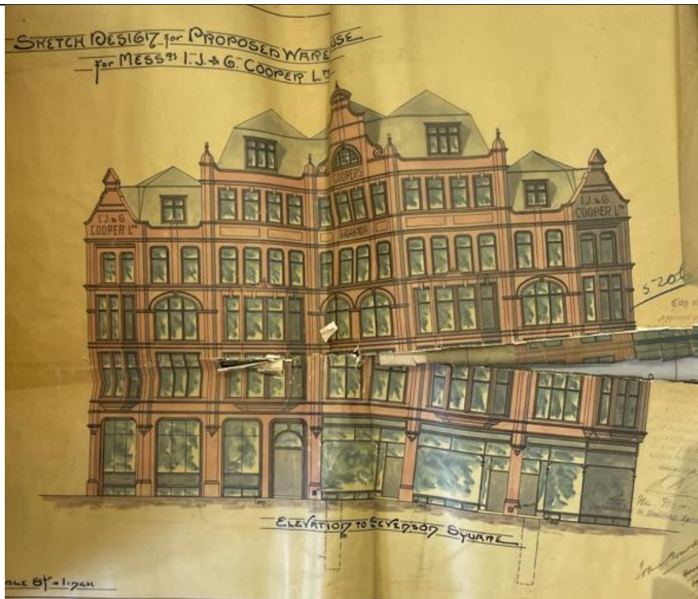
Figure 14: 1901, Elevation to Stevenson Square. The elevation to Stevenson Square presents four to five storeys, over basement. Built principally of red brick and terracotta, with polished marble and sandstone applied to the ground floor. The window treatment varies from floor to floor, with the windows to the ground floor being the largest and most open and the second-floor windows containing arched openings to every other bay. The ground floor units to Stevenson Square were fully glazed and open to the square, providing these were designed as shopfronts.
