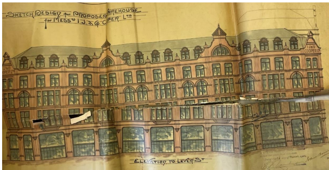
Figure 15: 1901, Elevation to Lever Street. The elevation to Lever Street presents four to five storeys, over basement. Built principally of red brick and terracotta, with polished marble and sandstone applied to the ground floor. The window treatment varies from floor to floor, with the windows to the ground floor being the largest and most open and the second-floor windows containing arched openings to every other bay.
