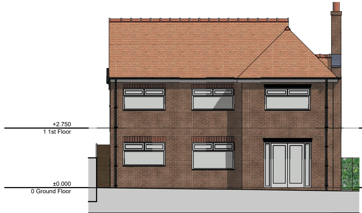
E-03 - North West Elevation 1:100
