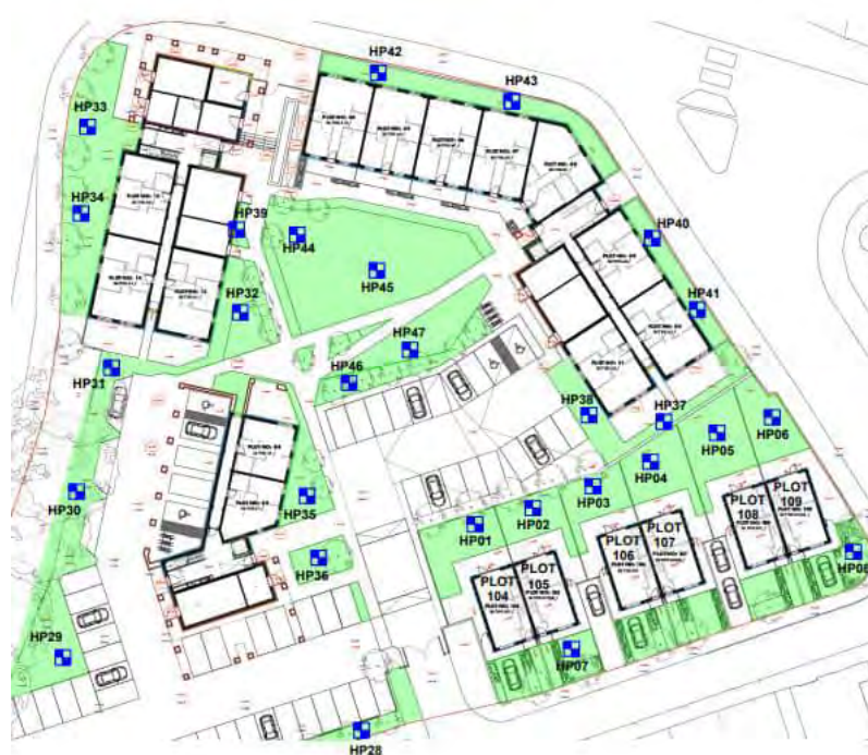
Figure 3 – Map showing the different areas of engineered landscaping on Site 2 (South).
