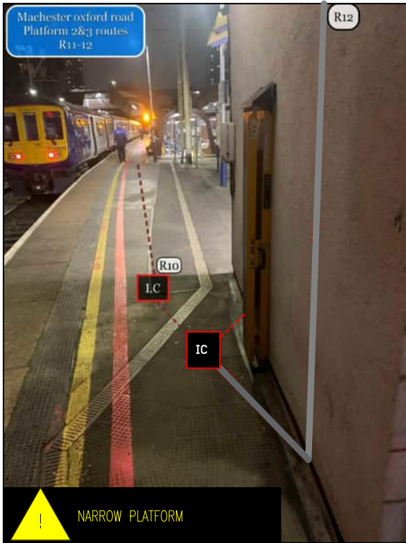
PHOTO 20 NEW SUB-DUCT AND INSPECTION CHAMBERS TO BE INSTALLED.
