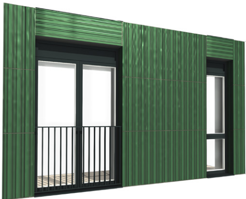
Typical Window Bay - Terracotta Tile and Reveal with Aluminium Soffit
