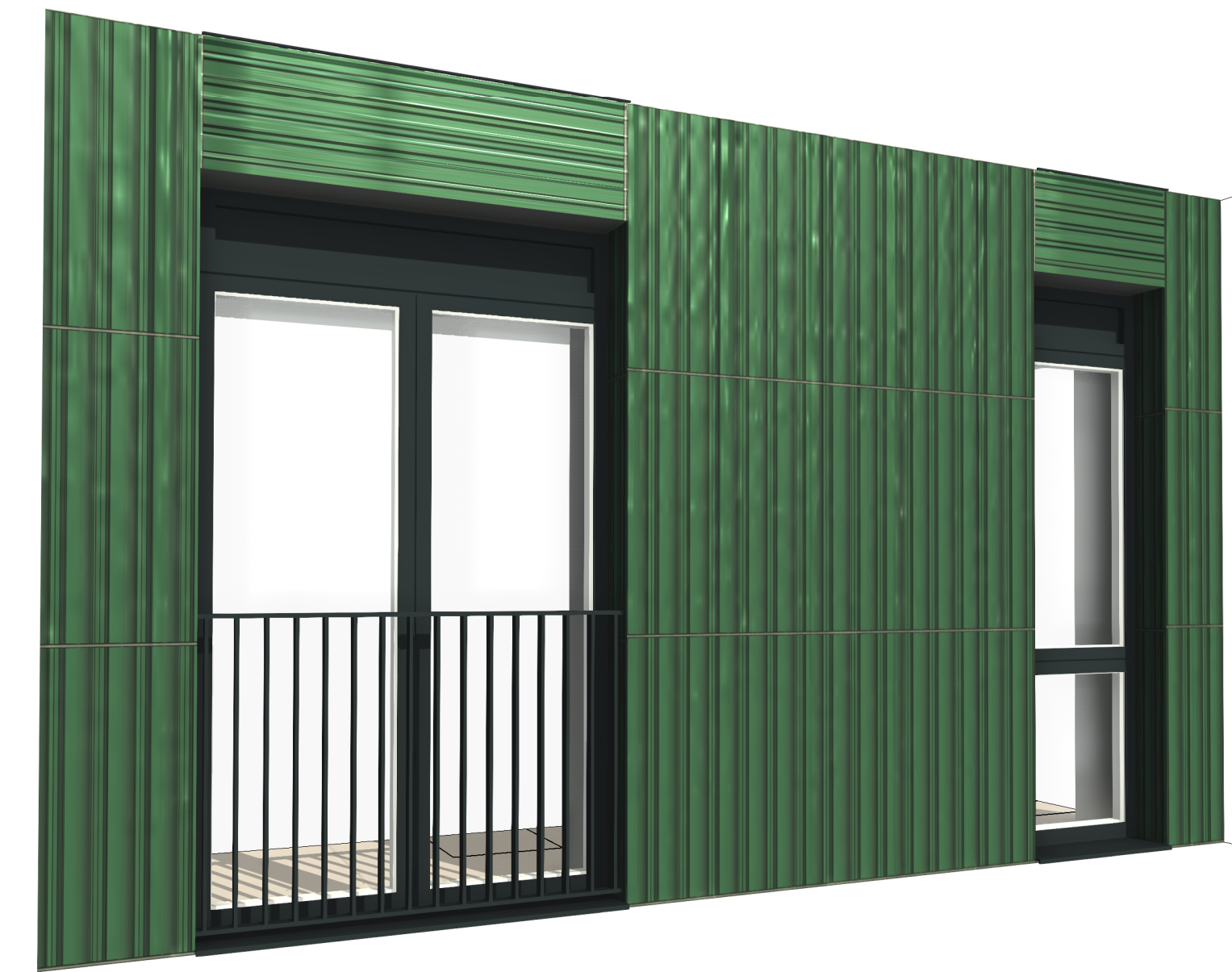
Typical Window Bay - Terracotta Tile and Reveal with Aluminium Soffit
