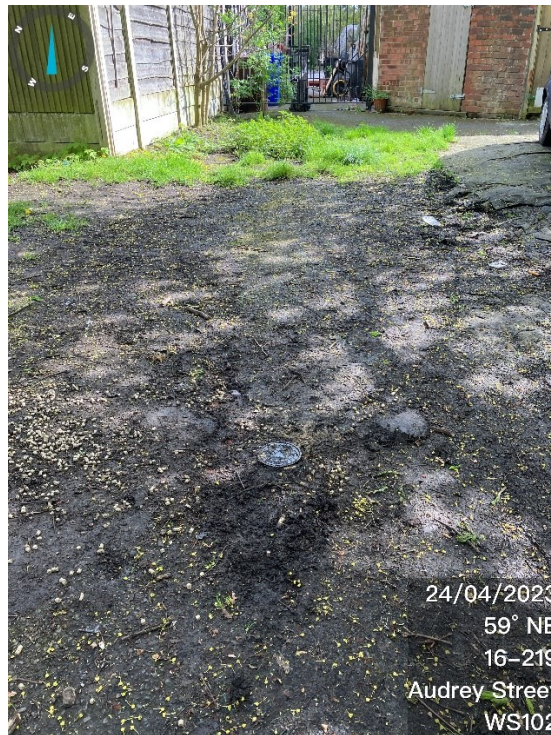
WS102 MONITORING WELL
