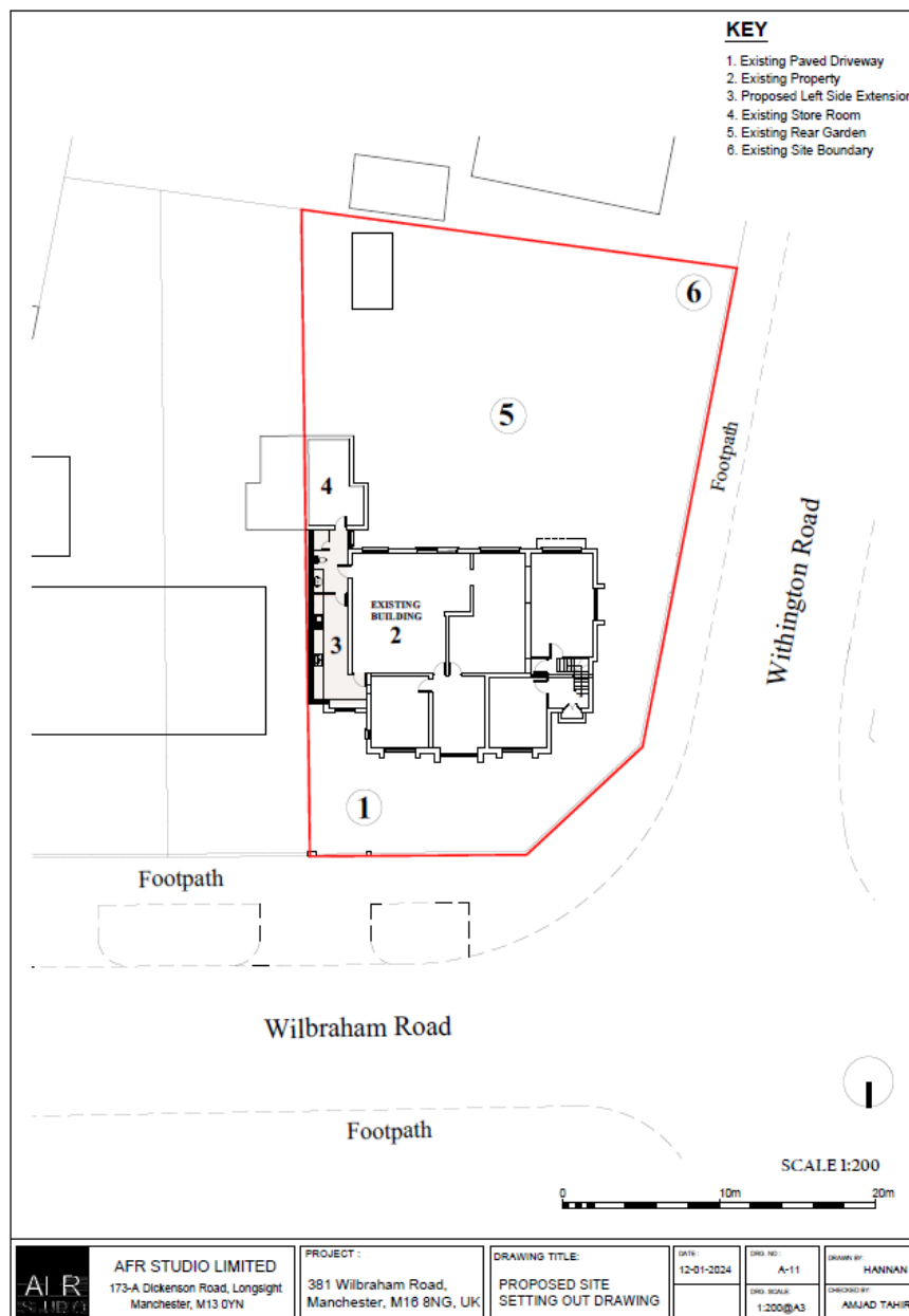
Figure 8. Submitted proposed site setting out drawing.
