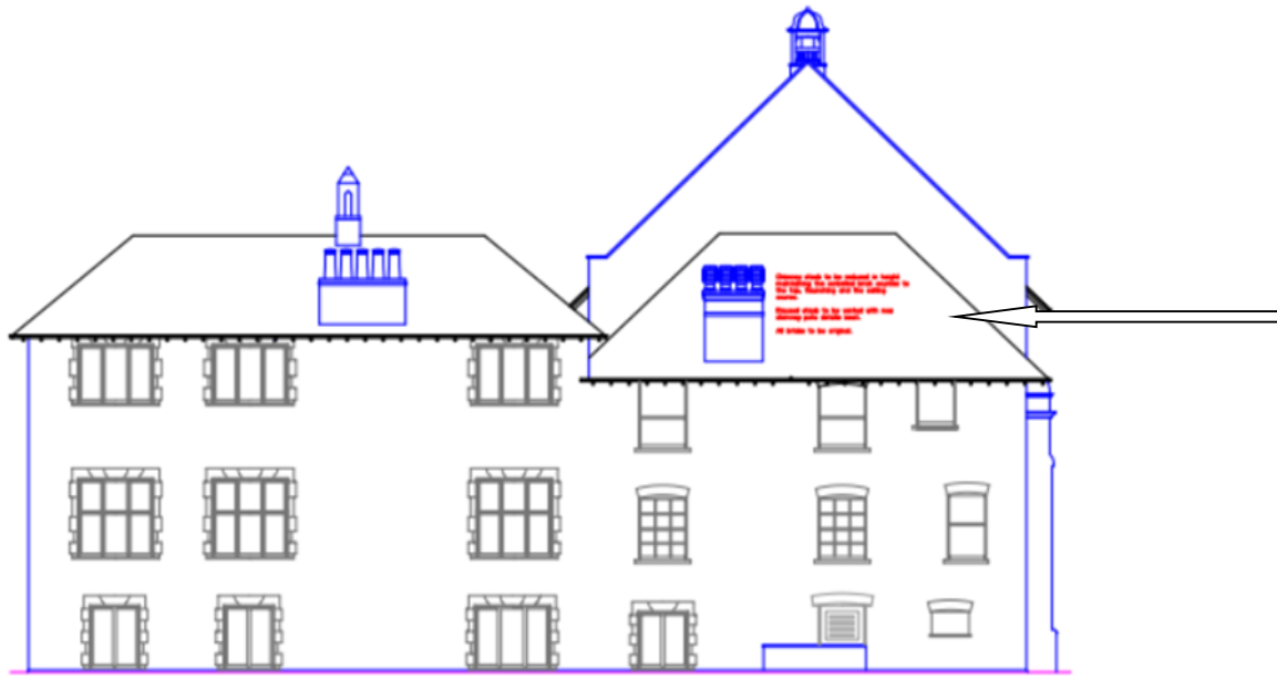
Proposed rear elevation showing reduced chimney stack
