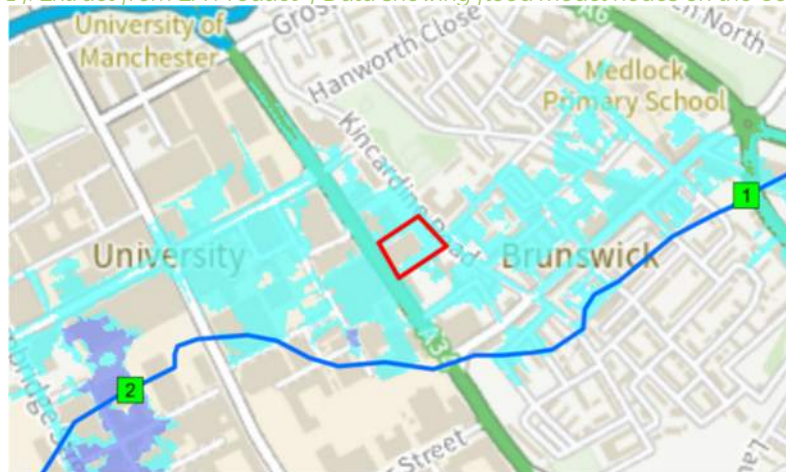
Figure 14: Extract from EA Product 4 Data showing flood model nodes on the Cornbrook
