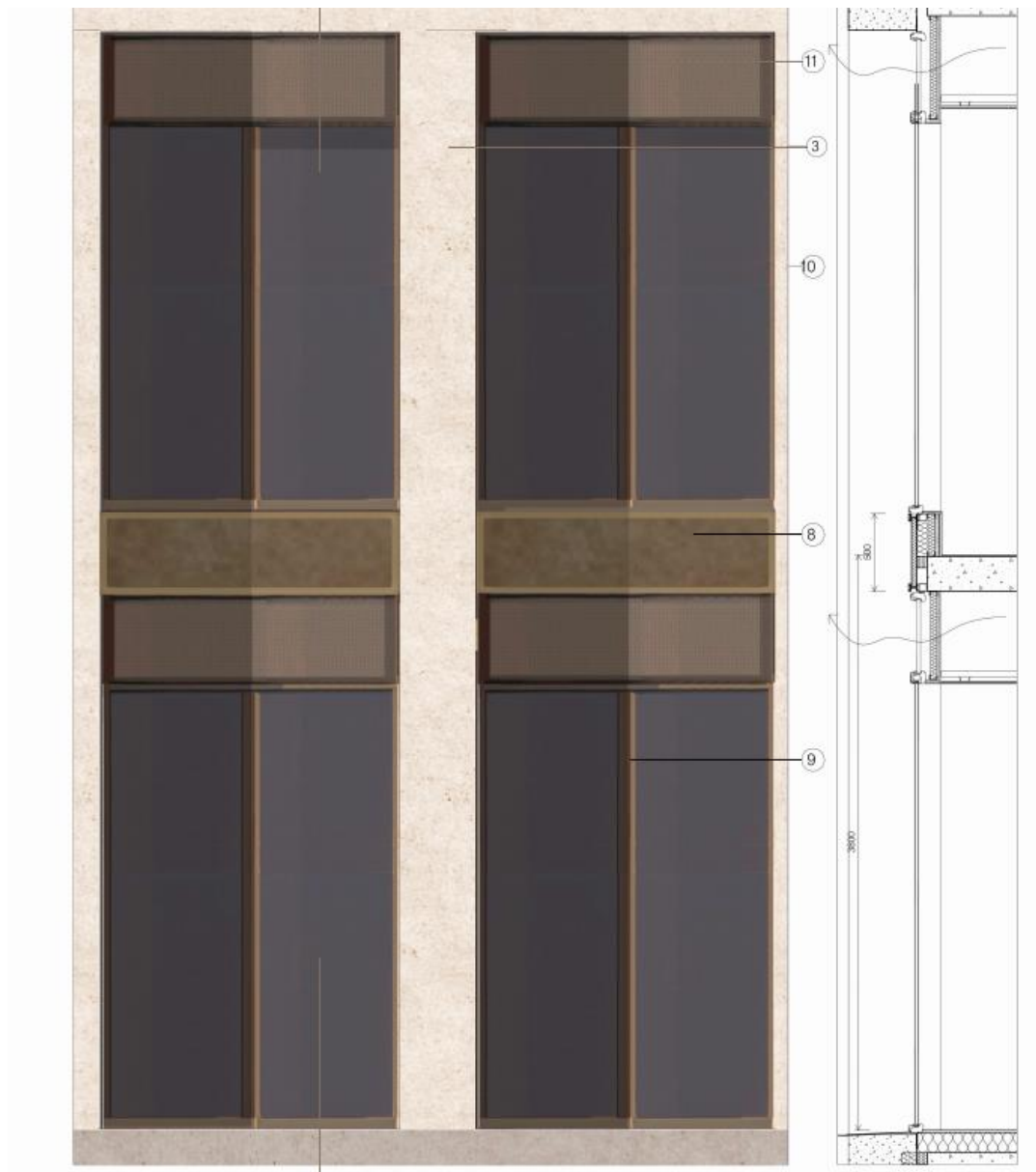
Typical Commercial Unit/Amenity Ventilation Panel Elevation
