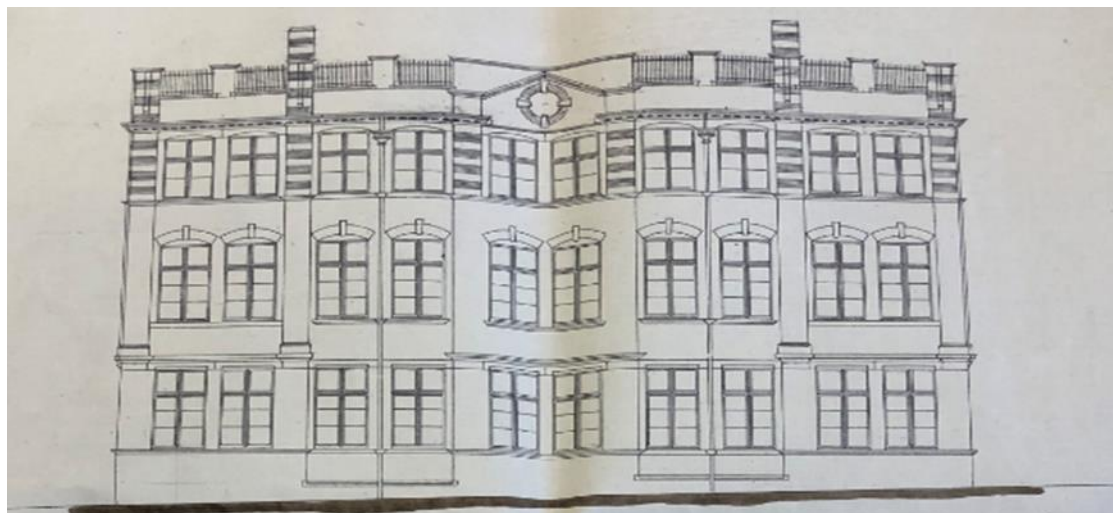
Figure 4: 1910 Proposed Great John Street elevation plan of the Atherton Street School, shown to have originally comprised only windows, with no doors. The large windows were designed to provide enough light to the double-height classrooms. (Source: Manchester Archives)
