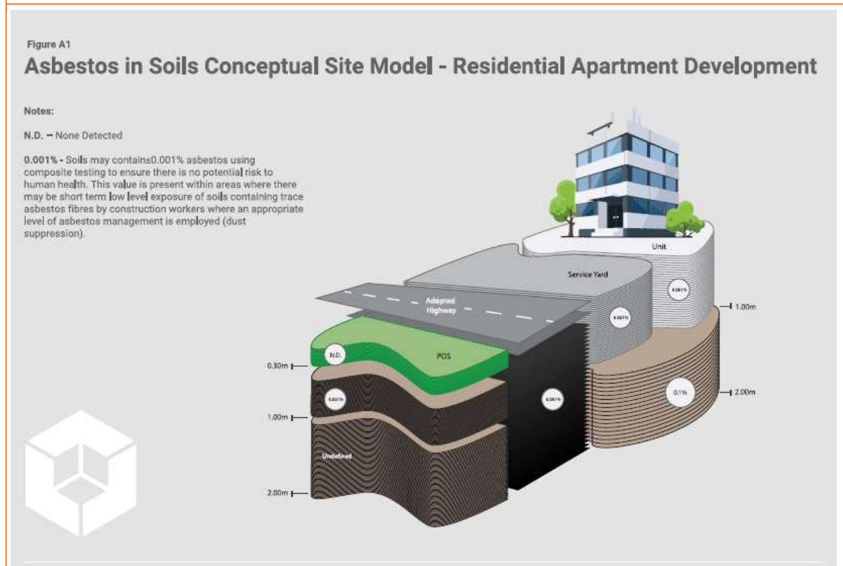
FIGURE 4.1 ASBESTOS RISK MITIGATION CONCEPTUAL SITE MODEL
