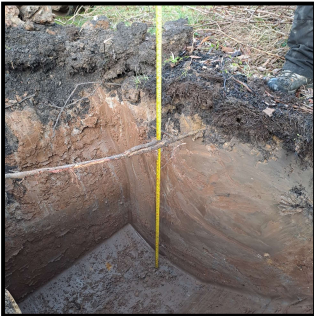
TRIAL PIT 2 – Clays at circa 0.30m below ground level.
