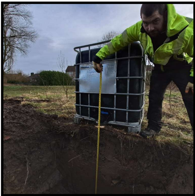
TRIAL PIT 3- Clays at circa 0.30m below ground level.
