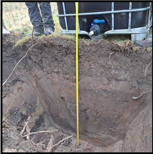
TRIAL PIT 1 – Initially sand turning to clays at circa 0.5m Below Ground level
