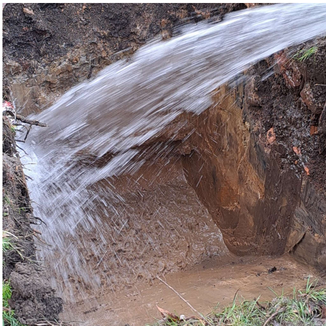
TRIAL PIT 4 Clays at circa 0.50m below ground level.
